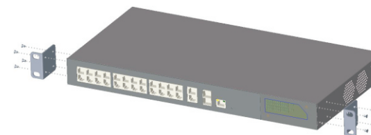
Figure 2-1 Install hangers diagram
